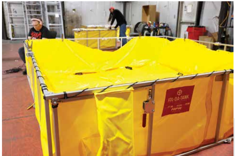
(Above) A folding frame tank is assembled at FOL-DA-TANK. These tanks are used by firefighters when fire hydrants are not available. It is collapsed and hung on a fire truck when not in use. (Below) Attachment pieces will be added to tanks so that a hose can be hooked up to the tank. Katelyn Metzger
